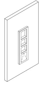
Surface mounting kit comes with (4) 1/4" spacers and (4) 3/4" spacers. Place the 1/4" Spacers on the outside of the frame first and secure to the frame. Stack on top of the 1/4" spacers the 3/4" spacers and secure to the frame. Surface mounting is complete.
