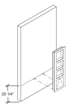
Place the inwall 20 1/4" above the finish floor, and fasten to wall through the back. (Block as needed by others)
